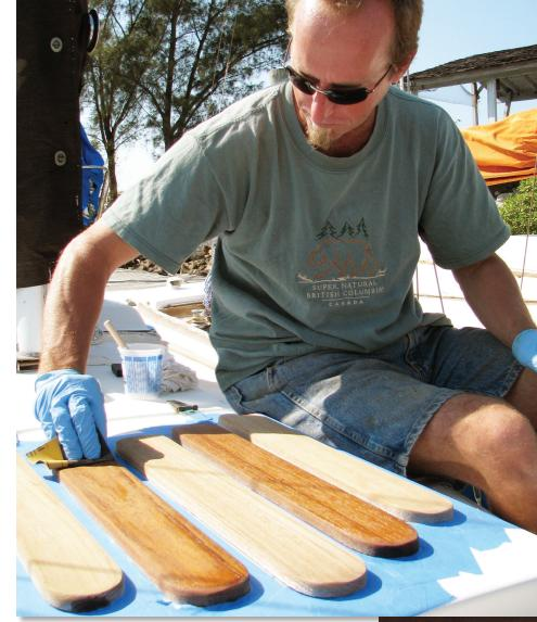
Of all the oils and sealers tested, Daly's Seafin was the only one that required sanding between coats. Here, PS tester Mike Collins wet-sands the Daly's as we launch a head-to-head test between it and a synthetic, Sikkens Cetol Natural, on this Cape Dory 25 in Sarasota, Fla. We'll be reporting on this and other longterm wood finishes tests in future issues.
